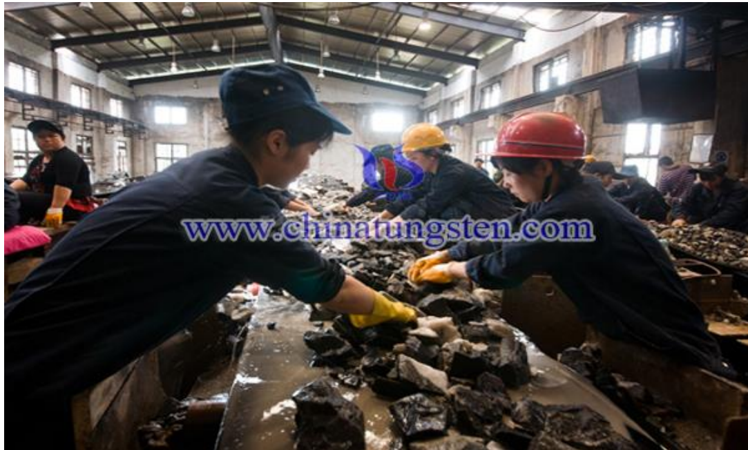
△Manual Separation Process of Traditional Tungsten Ore Development
